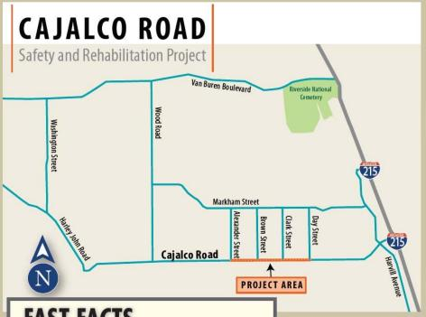
The project also includes new pavement, striping changes, new signage and relocating utilities. The traffic signals at Brown and Clark streets will be relocated and a new signal will be installed at Day Street. Bus stops will be added along with Americans with Disabilities Act (ADA) compliant sidewalks at the Clark Street intersection.
